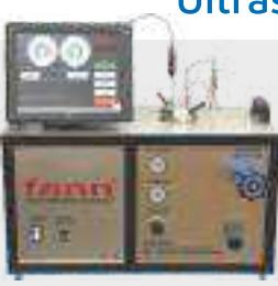
An ultrasonic compressive-strength test is used to help plan a cementing schedule for a well.
