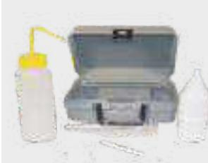
A simple, accurate and inexpensive sieve analysis apparatus for determining the sand content of drilling muds.
